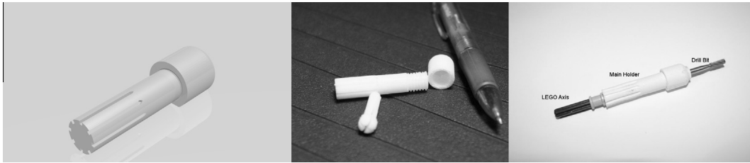
Fig. 2. The 3D design of the chuck (left) and the 3D printed one (right).
